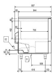
Drain Electrical inlet (power) ΕI Refrigerant Outlet
